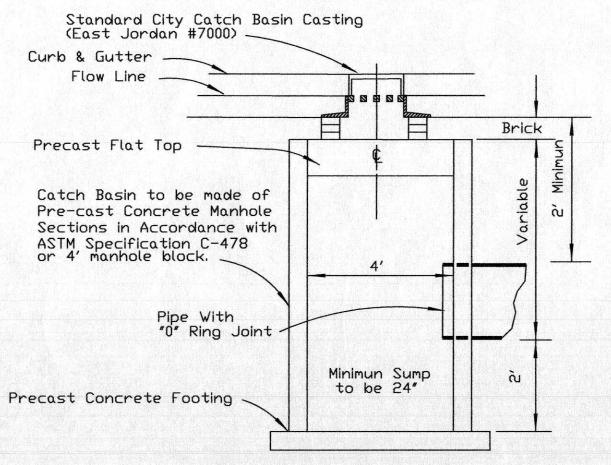
The top of Pre-cast Cone shall be sufficiently below ground elevation as shown on plan to allow for the adjustment of Catch Basin casting with either brick or block.
